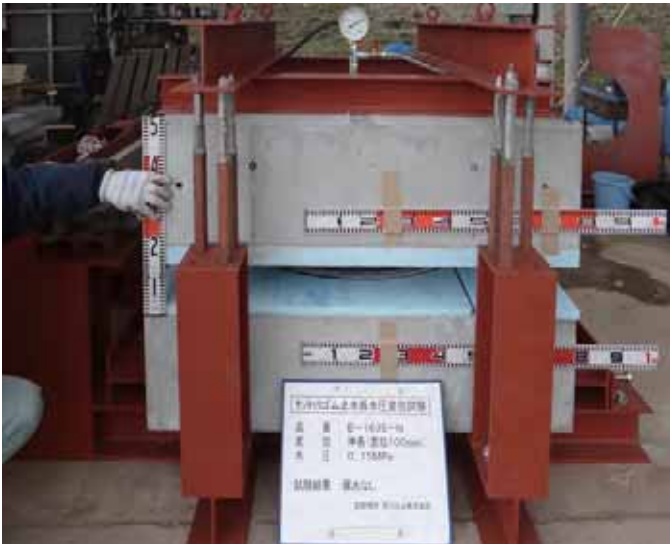
伸び量100mm/耐水圧0.15MPa
