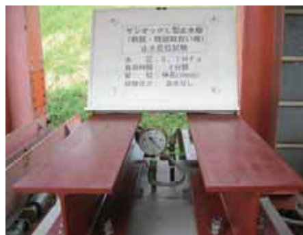
伸び量30mm/耐水圧0.1MPa
