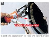
Insert the expansion jig into the jig insertion slot and tilt it slightly to the right toward the drilling center.
